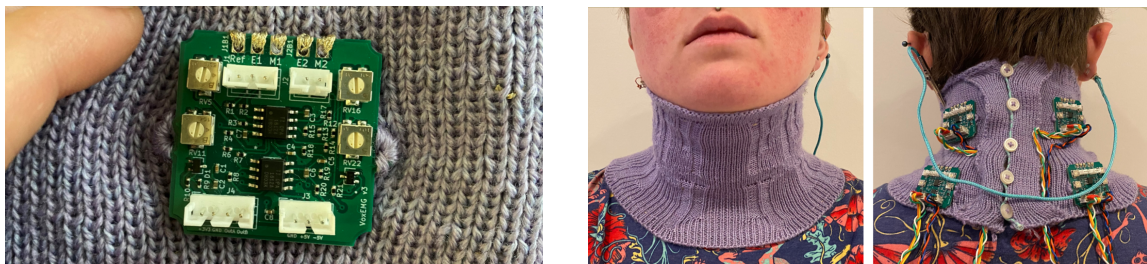
(a) The VoxEMG board developed for sensing activation of the laryngeal muscles.
